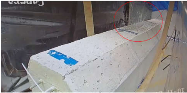
Figure 10. Concrete body after Mini-Frac test
